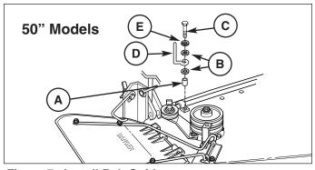
Figure 7. Install Belt Guide
